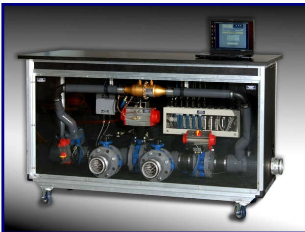
Test Console Automated control of air-water-structural and cycling tests
